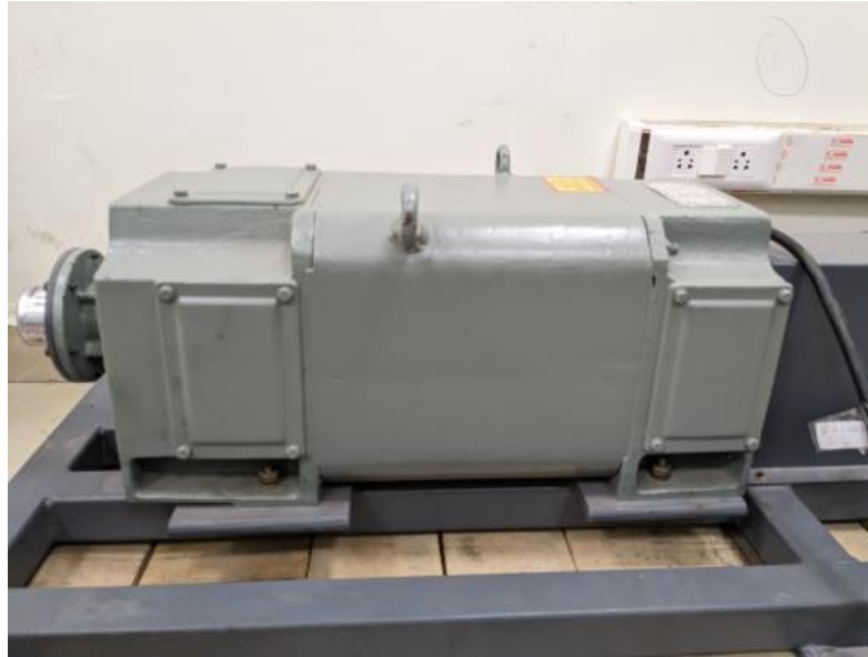
Figure 5. 26 DC machine used for wind emulation in the laboratory setup
