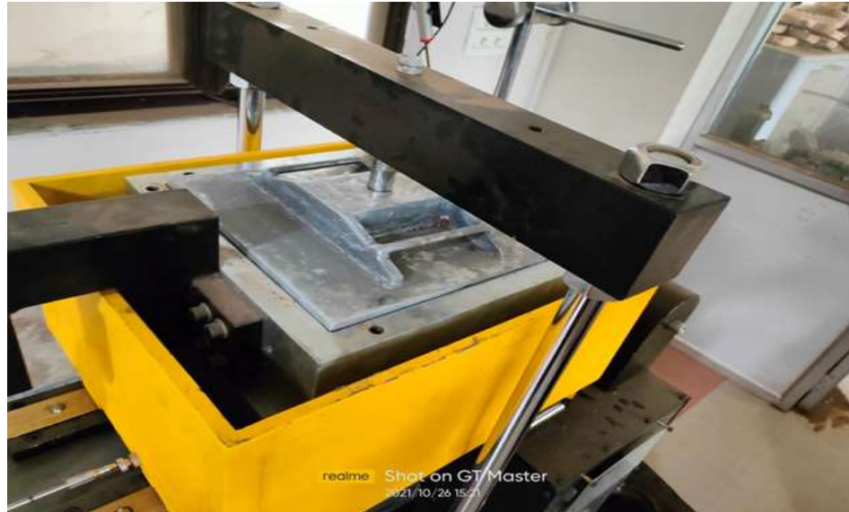
Figure 3.5: The Large shear Box setup used for the experimental study
