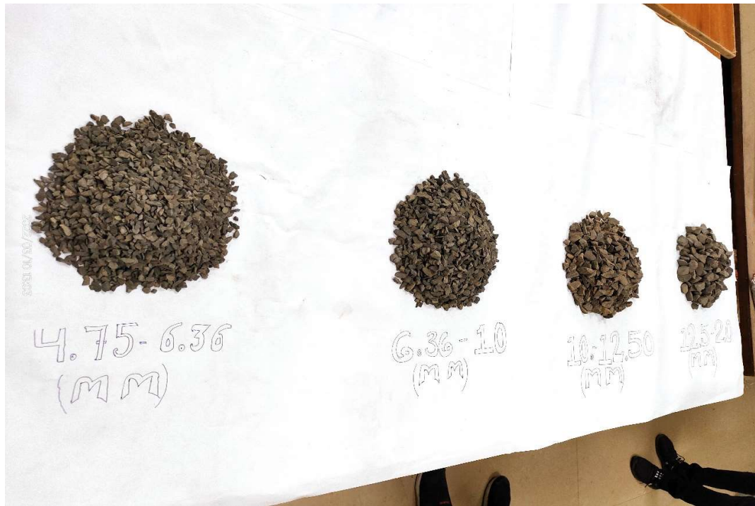
Fig 3.3: Aggregate samples prepared for infill material of (a) 50 mm, (b) 75 mm diameter, (c) 100 mm, (d) 150 mm
