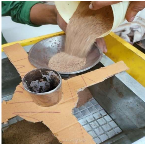
(b) Sand filling without compaction
