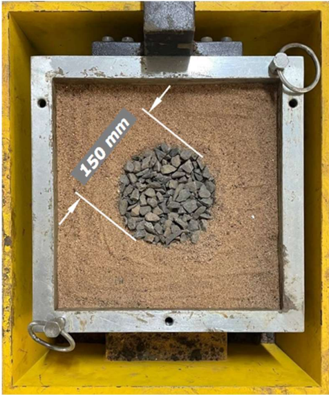
Fig 3.9: - Ordinary Stone Column installed in the sand bed
