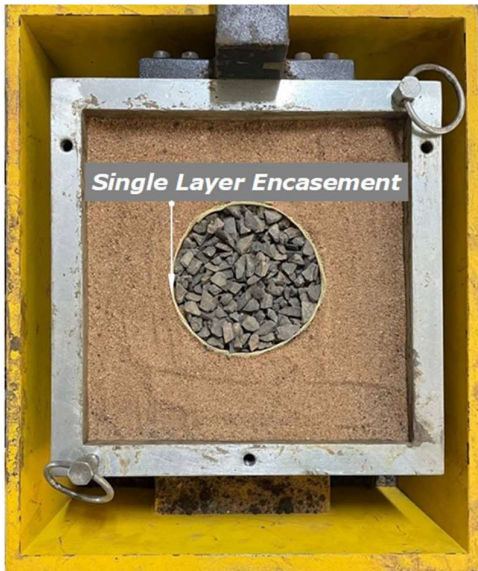
Fig 3.10: - Single Layer Encased Stone Column installed in the sand bed
