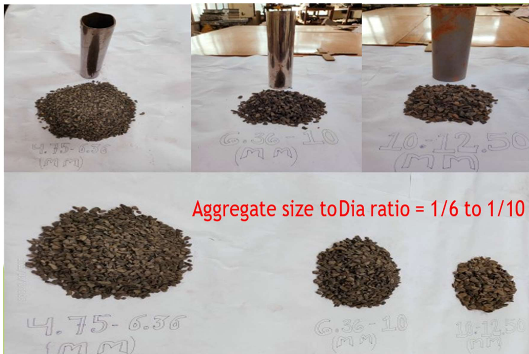
Figure 3.1: Particle size distribution for sand and aggregate samples
