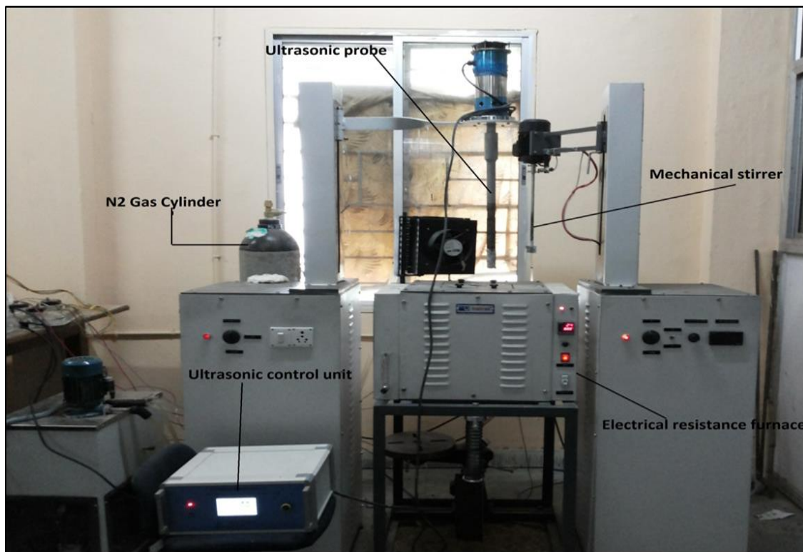
Figure 4.2: Stir Squeeze casting assisted with ultrasonic transducer
