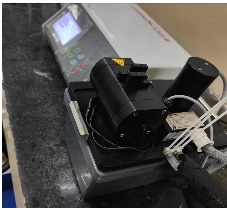
Figure 4.5: Twin Jet Polishers (Struers)
