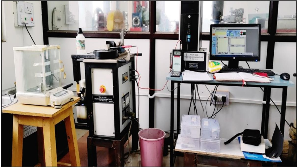
Figure 4.13: Pin-on-disk wear setup (at the Material testing lab, MANIT)
