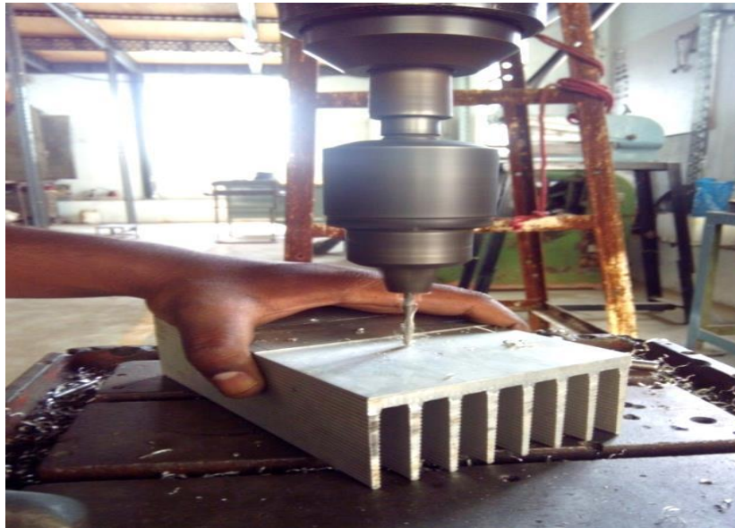
Figure 3.9: Drilling for creating holes
