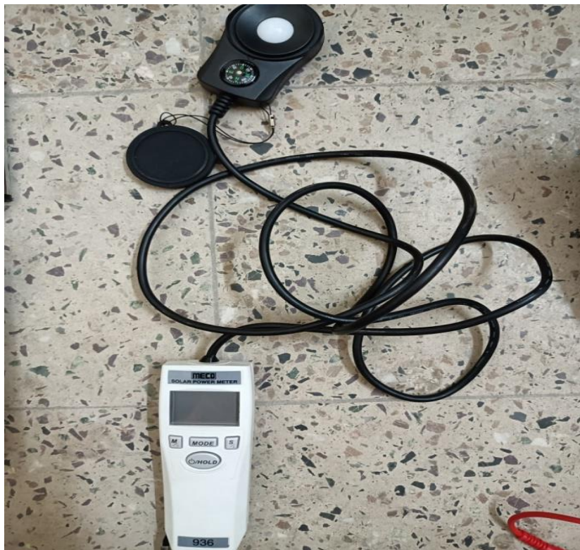
Figure 3.21: Solar power meter
