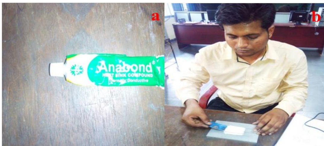
Figure 3.14: Anabond paste and pasting modules on the absorber
