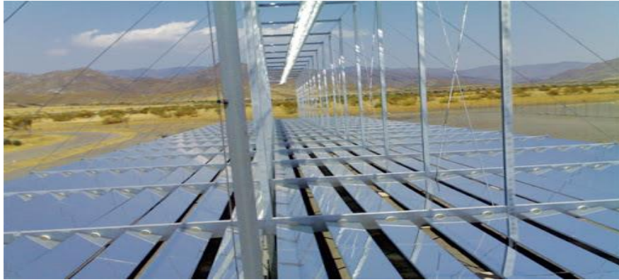
Figure 2.19: Linear Fresnel lens reflector [180]
