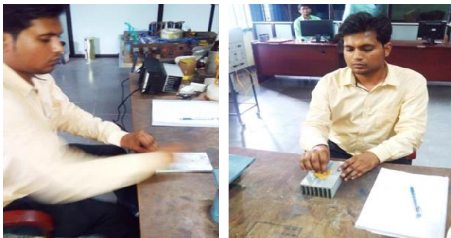
Figure 3.12: Smoothening of surface of heat sink & absorber plate
