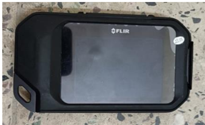
Figure 3.22: Thermal camera (FLIR C3-X)
