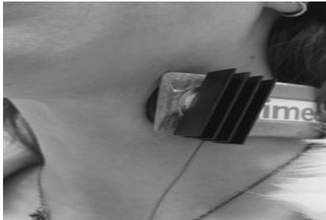
Figure 2.25: Extracted heat from body utilized in TEG [191]
