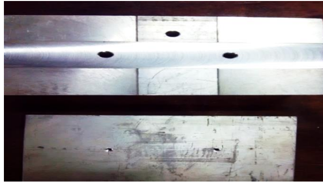
Figure 3.11: Heat Sink & absorber Plate ready, after milling process
