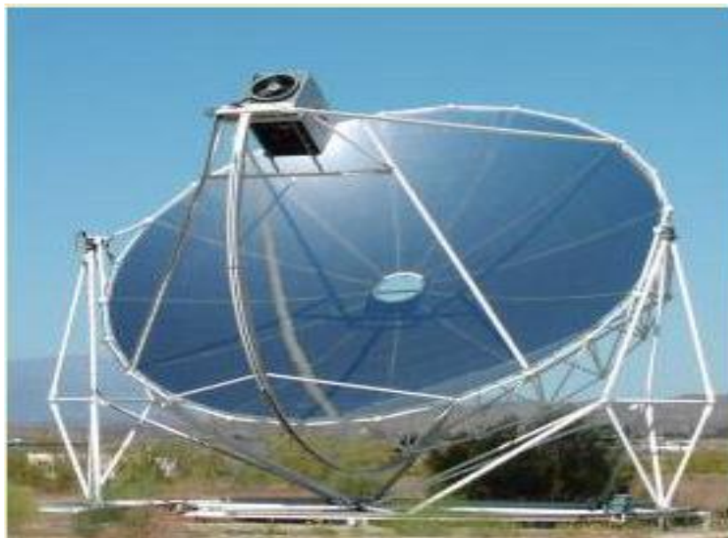
Figure 2.17: Parabolic dish solar concentrator [179]
